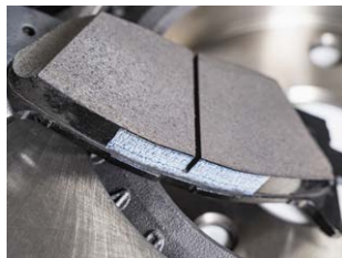
Brake pad containing aramid as a filler
